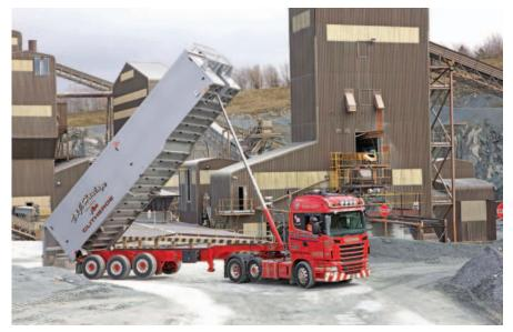
competitive equipment. Working with a new Scania R440 6x2 Hi-Line tractor unit, the Wilcox/Hyva trailer offers a 29,750kg payload. The tractor was built on the
